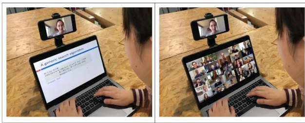
Figure 3. Our cheap simple hack for telepresence.
