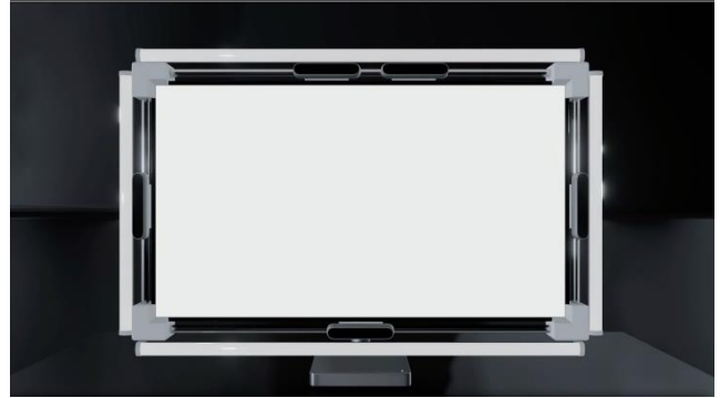
Figure 1. A CGI rendering of the frame around a display. The final system included four cameras.
